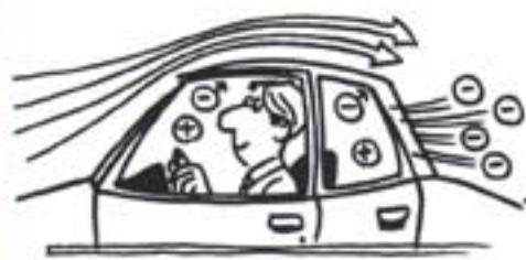
Air friction knocks electrons off the car's metal body.
